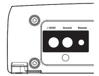
The A2150's "+12VDC" and "Ground" connections are designed to accept 8 AWG - 4 AWG power wire. 8 AWG is a minimum power wire size for this amplifier.
